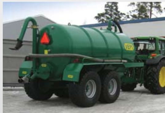
A 15,100 litre vacuum tanker model with the following accessories: 12 m drip hose system; sprung bogie unit with a mechanically controlled rear steering axle; 700/50R26.5 tyres; 12m 3 /min compressor; precipitation container; oil receiver for exhaust air from the compressor; needle gauge; hydraulic-powered filling hole; hydraulic-powered closing valve for spreader pipe; down fill combination; lift coupling.
