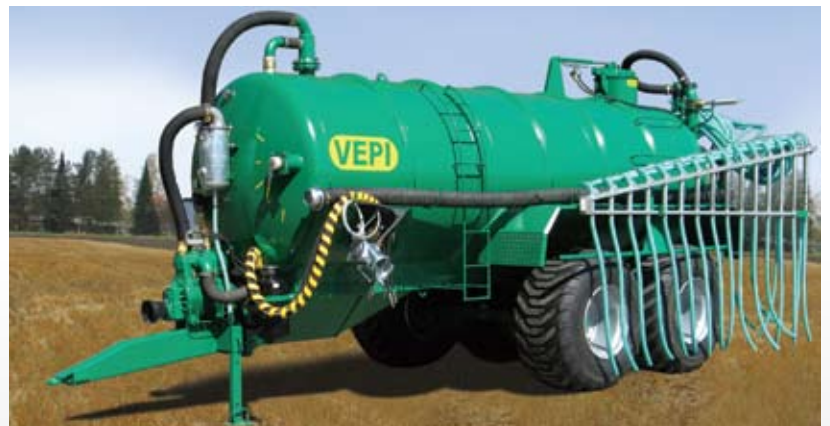
A 15,100 litre vacuum tanker model with the following accessories: 12 m drip hose system; sprung bogie unit with a mechanically controlled rear steering axle; 700/50R26.5 tyres; 12m 3 /min compressor; precipitation container; oil receiver for exhaust air from the compressor; needle gauge; hydraulic-powered filling hole; hydraulic-powered closing valve for spreader pipe; down fill combination; lift coupling.
