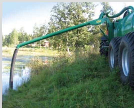
The vacuum arm is welded to the side of the tank. It ensures easy use and reach. The tank can be filled without leaving the tractor.
